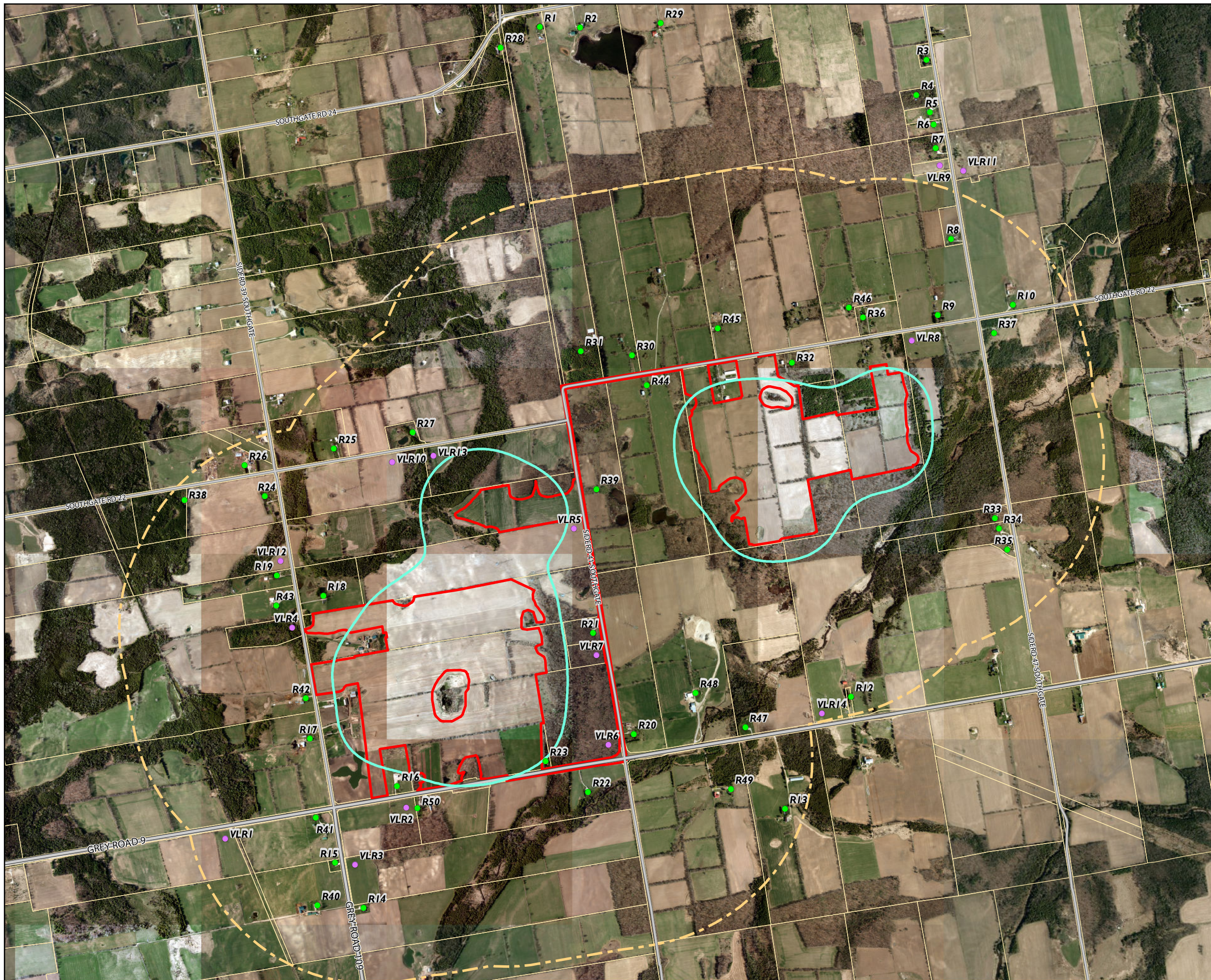
FIGURE 4 PREDICTED NOISE LEVEL CONTOURS AT 1.5 m HEIGHT
