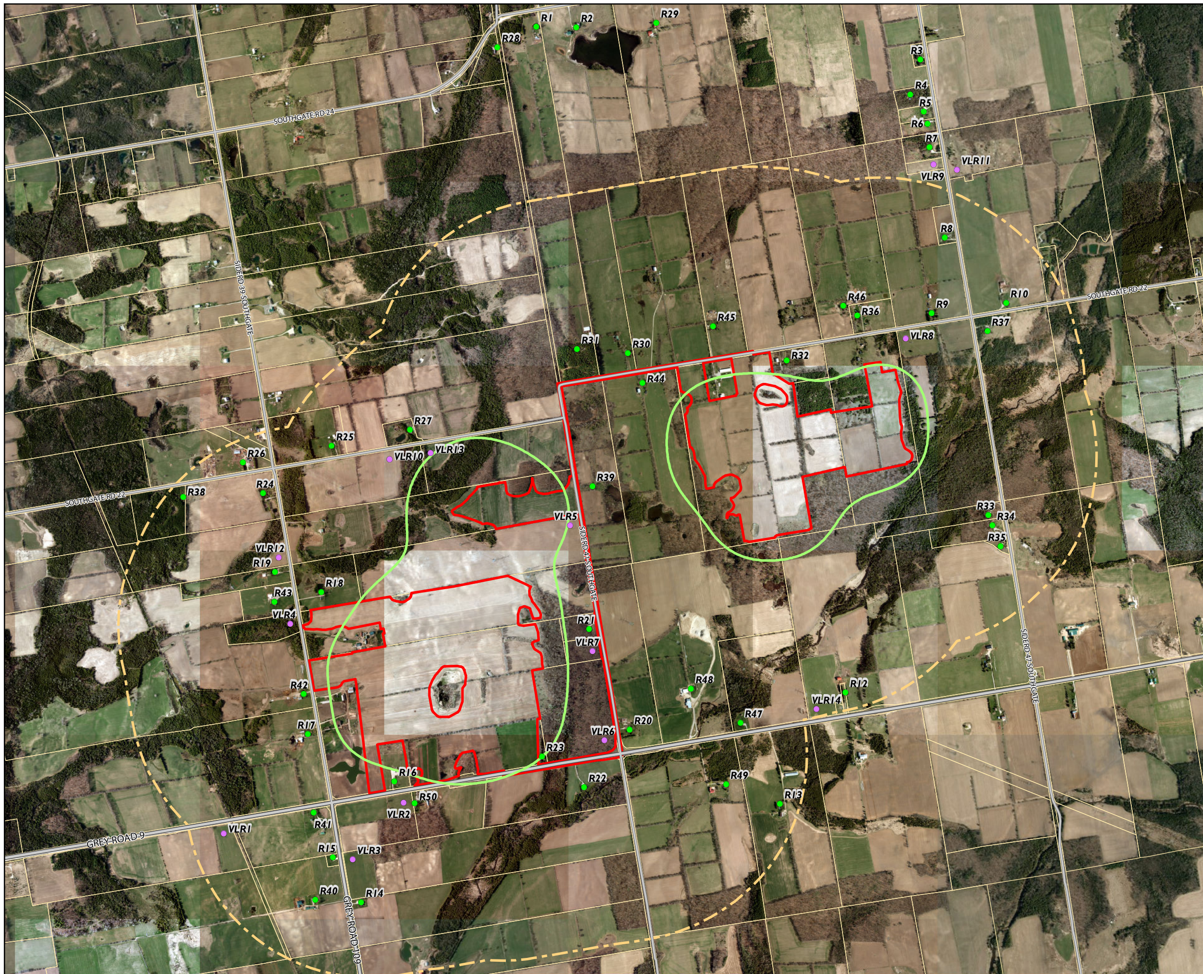
FIGURE 5 PREDICTED NOISE LEVEL CONTOURS AT 4.5 m HEIGHT
