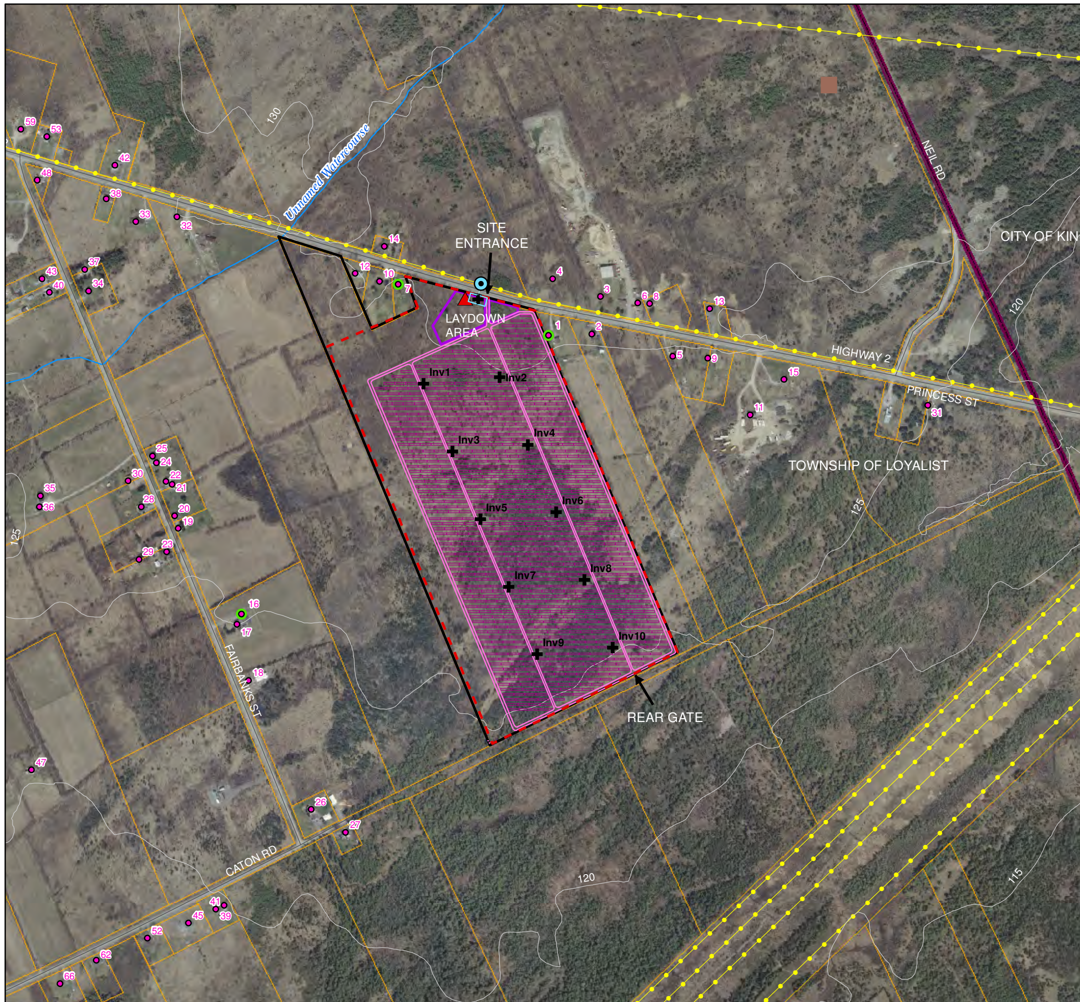
Figure 2.1 Axio Power Canada Inc./SunEdison Canada Kingston Gardiner Hwy 2 South Site Layout Plan HATCH™
