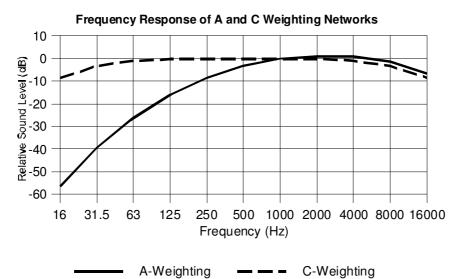
**dBC** - **Decibel, C-Weighted:** The logarithmic units associated with a sound pressure level, where the sound pressure signal has been filtered using a frequency weighting that mimics the response of the human ear to loud sound levels. C-weighted sound pressure levels are denoted by the suffix 'C' (ie. dBC). C-weighted levels are often used in low-frequency noise analysis, as the filtering effect is nearly flat at lower frequencies.
